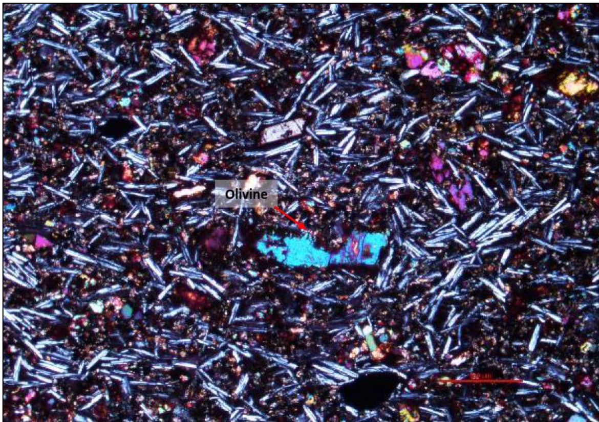
Plate 4 – Microphotograph displaying representative mineral assembly of the basalt including abundant plagioclase, fine tabular pyroxene and plagioclase with finely disseminated magnetite. Image shown in cross polarised light.
