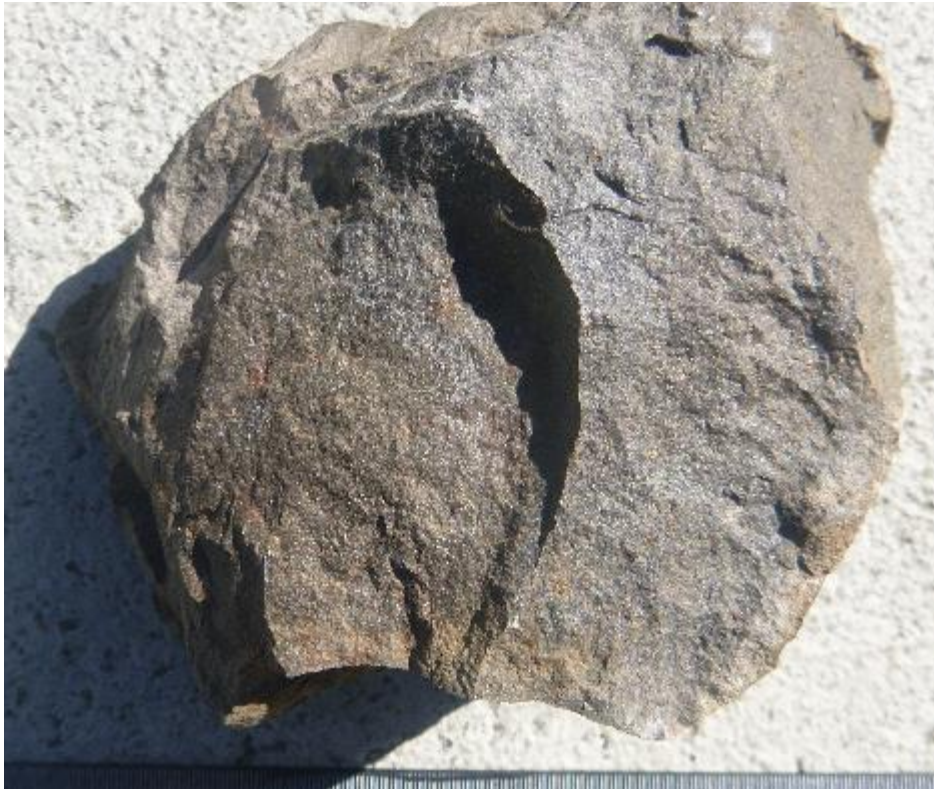
Plate 1: Photograph displaying weathered rind common among surficial spalls on-site. Vesicles in the basalt resulting from entrained gas bubbles remain as partially filled voids in the rock measuring to 0.5mm in diameter and hosting secondary quartz and ferruginous/argillic material.
